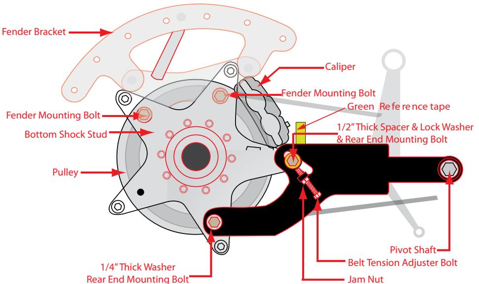
17. Attach fender brackets to fenders using supplied FENDER MOUNTING HARDWARE ★ *Note: side with more space from bolt holes to edge of fender goes toward the front.*
