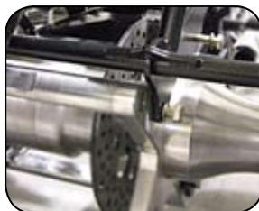
22. Install top two star plate bolts. Install lower mounting bolts and lock nuts on fender bracket. Install fender and fender bracket on other side as previously described.
