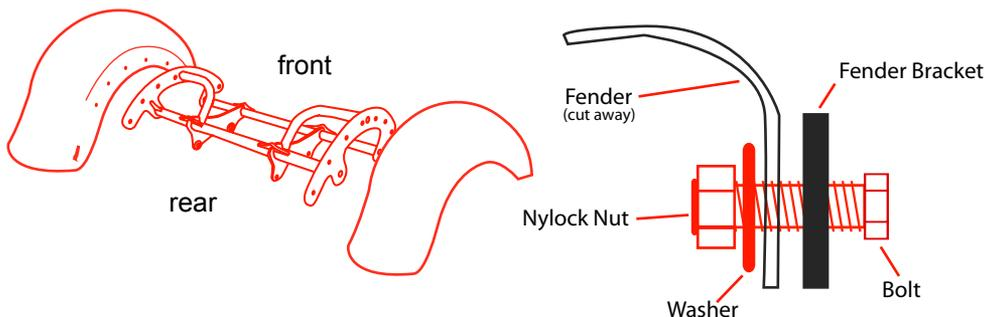
21. Remove two gold bolts on both sides. Install fender and bracket on the rear end.
