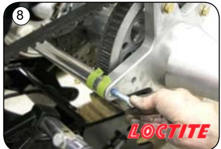
10. Install lower swing arm mounting bolts both sides, leave loose. Install upper swing arm mounting bolts, make sure to put the 1/4" thick washer between the swing arm and the star plate on both sides, leave loose. Refer to diagram for placement of washers and spacers.
