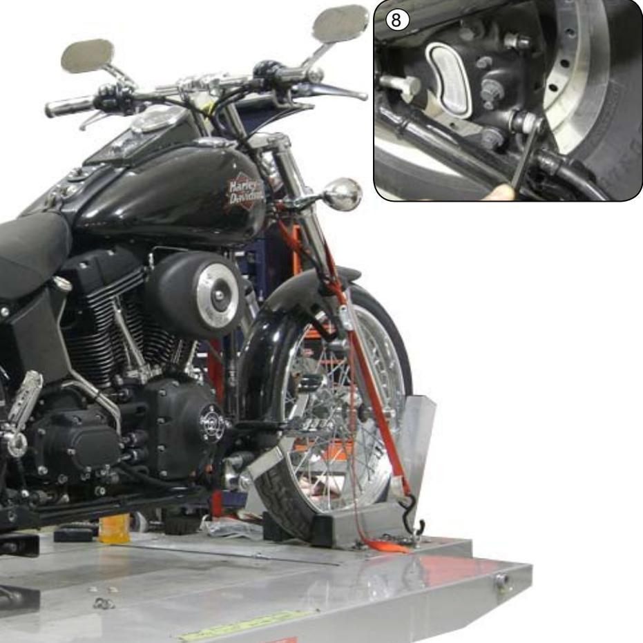
9. Remove wheel, splash guard and rear shock bolts. Remove swing arm pivot bolts. Remove swing arm.
